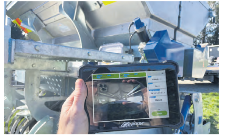
At the heart of the Boon seed drill is a waterproof, dustproof, and impact-resistant, wireless, rugged tablet that controls the machine. PHOTO SUPPLIED
